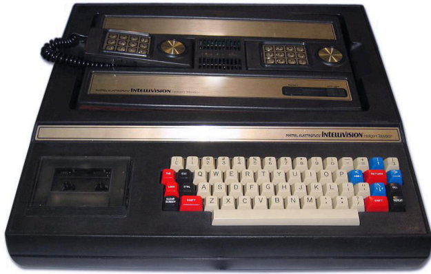
Fig. 7 - The Keyboard Component, which turned the Intellivision into a home computer (image: Daniel McConnell - source: Wikimedia Commons)
