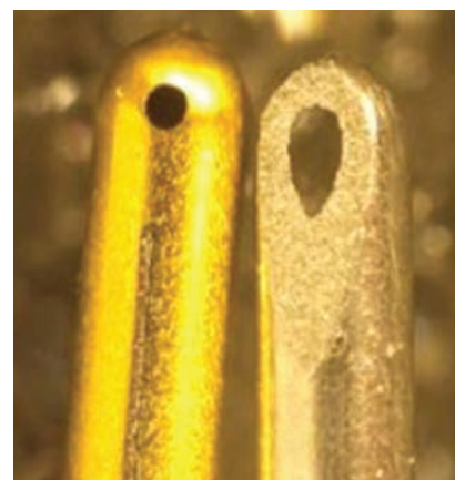
Figure 3. Examples of several tip designs for the hypersonic vitrectomy cutter. The single lumen design means the probe doesn't need to be straight, which allows flexibility in the shapes of the tips that can be created.
