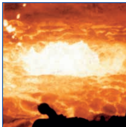
Gas Purging in an Electric Arc Furnace
