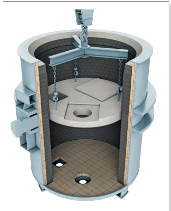
Figure 9. Installation of an IBOS shape into a ladle using lifting connections.
