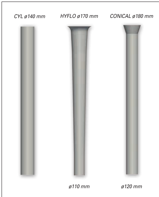
Figure 11. Simulated taphole geometries. (a) cylindrical (CLY) with a diameter of 140 mm, (b) HYFLO with a transition from an inlet diameter of 170 mm to an outlet diameter of 110 mm, and (c) cylindrical with a conical entrance area (CONICAL) decreasing from an inlet diameter of 180 mm to 120 mm.
