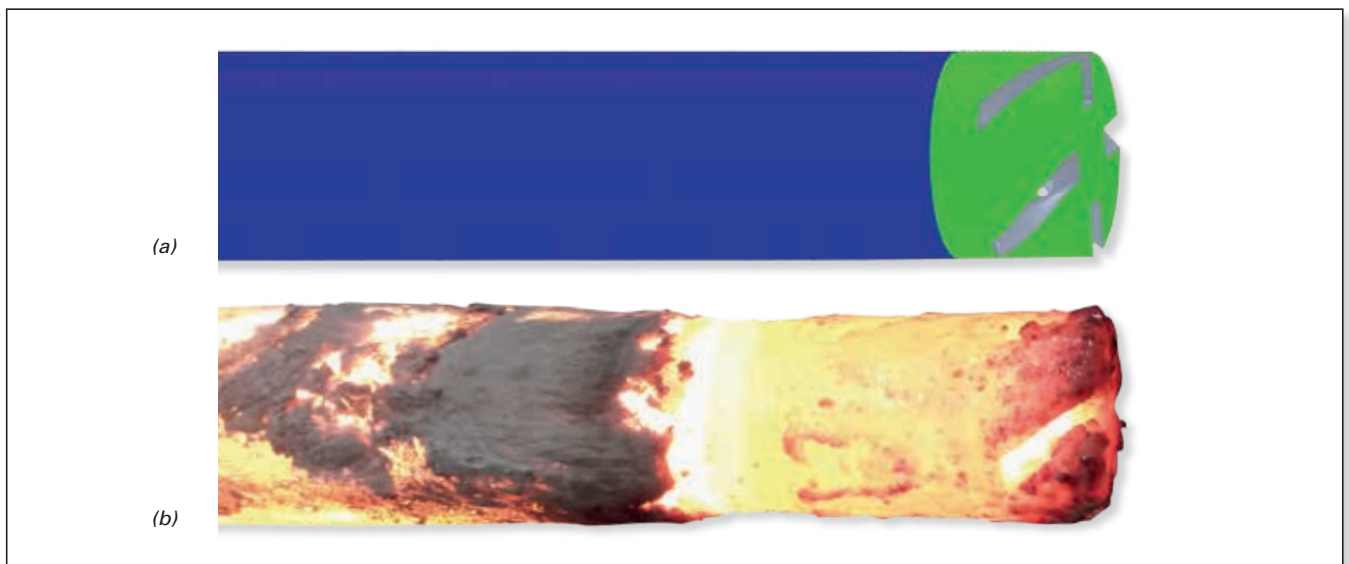
Figure 10. (a) schematic showing the original GYRO Nozzle geometry and (b) appearance of a GYRO Nozzle after use.
