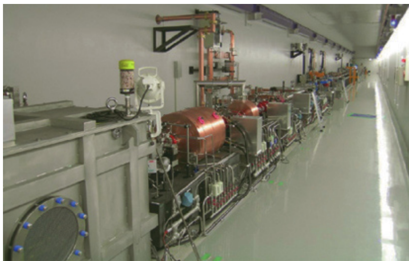
Figure 1: A view at the beam hall of the FEL test facility. The electron gun is contained in the grey box on the left.
