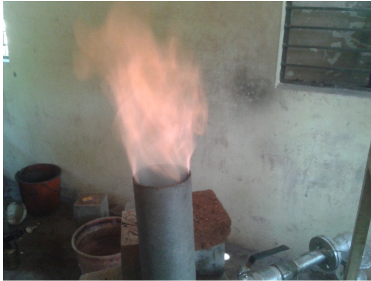
Figure 2: Flaring of PG in a burner
