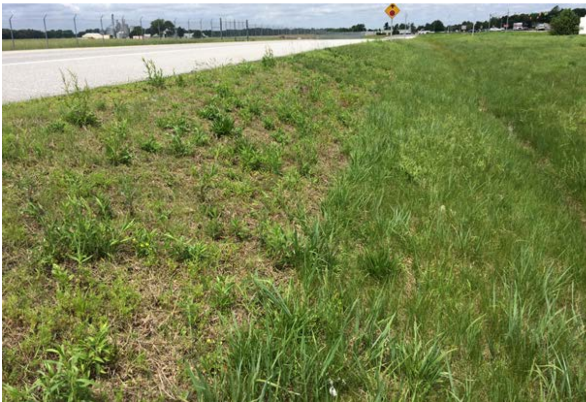
Figure 13. Plots at the Eastern Shore site in 2018. Although fescues established well in 2017 and reduced initial weed abundance, the site became increasingly invaded by weeds throughout the project. Fescues never reached a height that required mowing.
