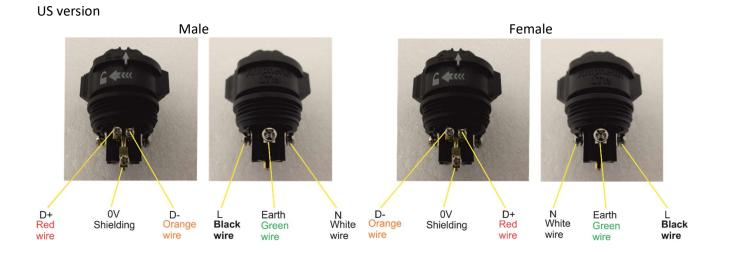
4. After connecting wires to the connector, tighten the three data wires (D+,D-, 0V) by means of the cable binder (6).
