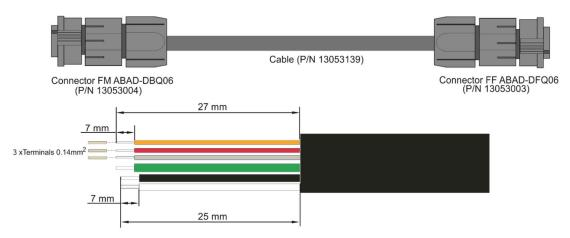
3. Put parts of the connector on the cable (5) and connect wires to the connector. First connect power wires (L,N, Earth) and after that data wires (D+, D-, 0V). Avoid excessive torsion of data wires!
