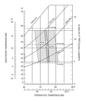
Fig.4 ASHRAE Comfort Chart Modified for Radiant Heating (Ref. Ch. 16 - 1987 ASHRAE HVAC System & Application Handbook)
