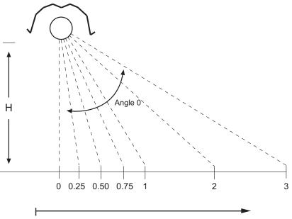
Horizontal distance from centerline of burner emitter at floor level (in multiples of H).
