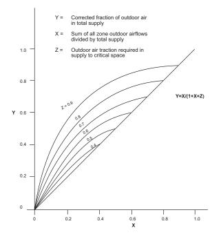
Fig. 3 Ventilation Reduction in Multiple Spaces Supplied from a Common Source
