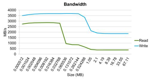
Please refer to diagram below for memory partial read, partial write and partial read/write bandwidth results.
