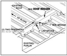
Figure B – Lap for Special Roof Hugger – (16 & 14 GA Purlins)
