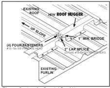
**Figure C –** Lap for Special Roof Hugger – (12 GA Purlins)
