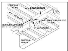
Figure A – Lap for Standard Roof Hugger – (All Purlin Gauges)
