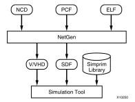
The FPGA Timing Simulation flow uses the following files as input:
