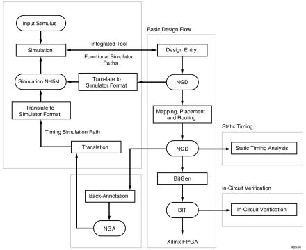
The following figure shows the verification methods of the design flow for CPLDs.
