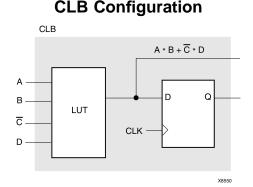
Observe that MAP has generated an active low (C) instead of an active high (C). Consequently, the Boolean output for the combinatorial logic is incorrect. When you run NetGen using the mapped.ngm file, you cannot detect the logical error because the delays are back-annotated to the correct logical design, and not to the physical design.
