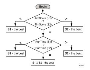
Starting with 12.1 software, you can use the **-pwo** option to run XPower Analyzer and calculate the total power dissipated by the design. If you enable power analysis, power data will be taken into account for selecting the best strategy. The following diagram illustrates the best strategy selection algorithm:
