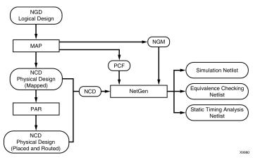
NetGen can be described as having three fundamental flows: simulation, equivalency checking, and third-party static timing analysis. This chapter contains flow-specific sections that detail the use and features of NetGen support flows and describe any sub-flows. For example, the simulation flow includes two flows types: functional simulation and timing simulation.
