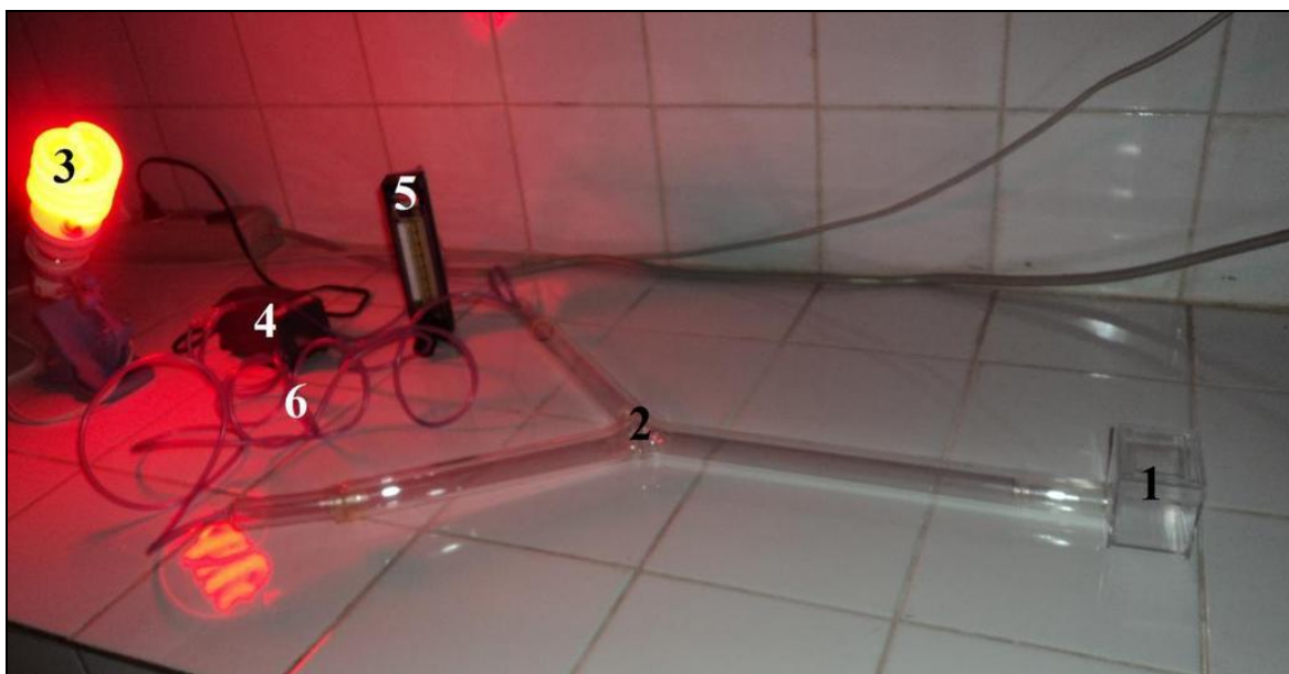
Fig.1. Bidirectional olfactometer "Y" shaped tube (Masna, 2016)
