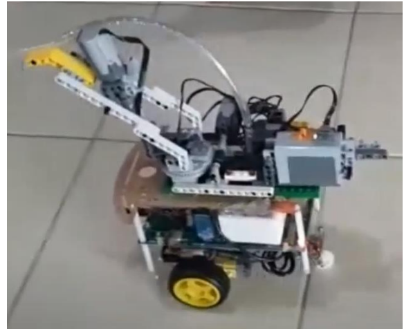
2Fire extinguishing robot built by Kaukab students
