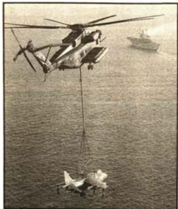
ONE of HMS Invincible's Sea Harriers gets a lift back to the carrier thanks to a US Navy Sea Stallion helicopter. The Harrier had suffered engine trouble and diverted to land at an Italian airfield.
