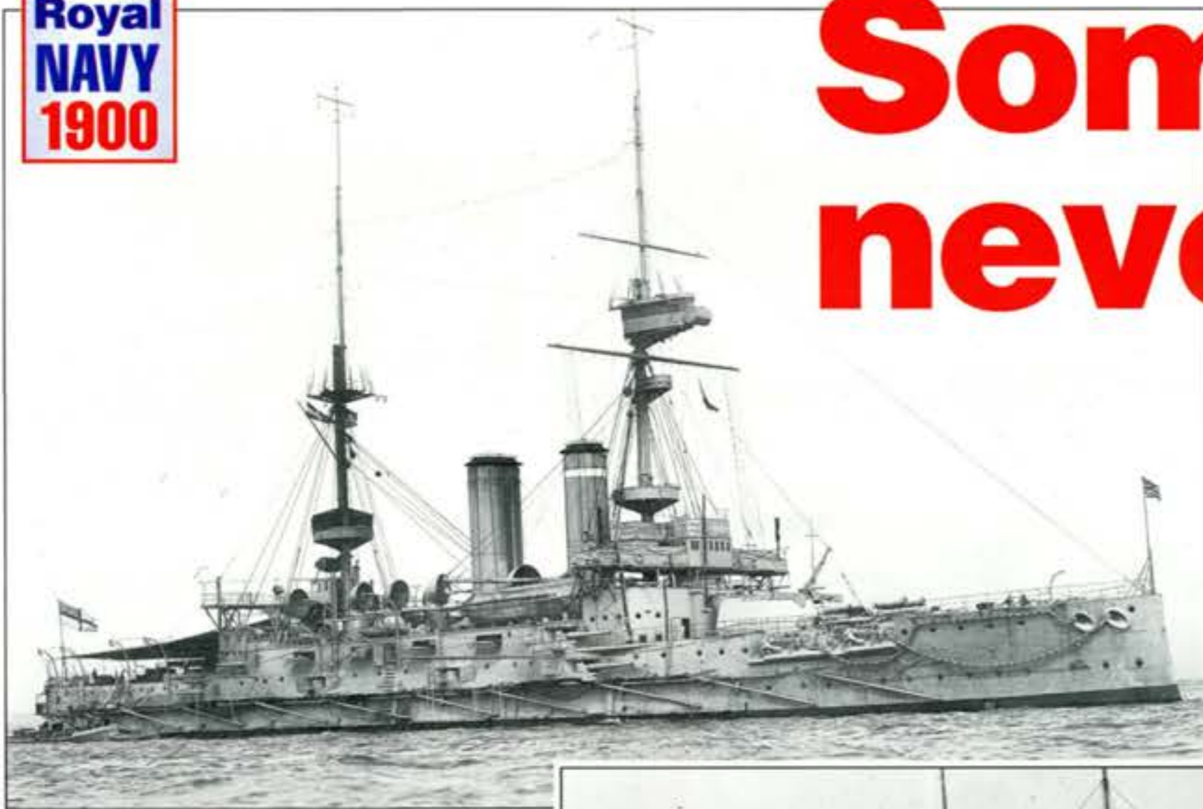
NEW CENTURY, NEW SHIP: The battleship HMS Implacable (above) was designed and built at the end of the 19th century and represented the modern face of the Royal Navy at the end of the Victorian era. A pre-Dreadnought of the Formidable class, she cost just over £1 million to build at Devonport, where she was launched in March 1899, and displaced around 15,000 tons. Her main weapons were her four 12in guns, supported by 12 6in guns and 18 12-pdrs, although in 1916 she had four 6-in guns and eight 12pdrs removed. Implacable, with her complement of 780, spent much of her early life in the Mediterranean, although she twice suffered serious technical faults – in 1905 a burst steam pipe killed seven, and a boiler exploded the following year. Her war service took her from the Channel to the Dardanelles and Adriatic, the East Indies and Egypt, and having survived the war with Germany it was ironic that she was sold in 1921 and broken up in that country. Picture: Royal Naval Museum, Portsmouth
