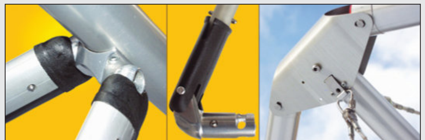
Fex details from left to right: A-frame attachment with high-tech fittings, aerodynamically shaped A-frame corner and Perunal nose plate.
