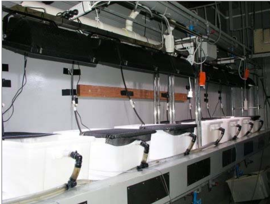
Photo 1: Aquarium setup for long-term growth of corals at controlled environmental conditions.
