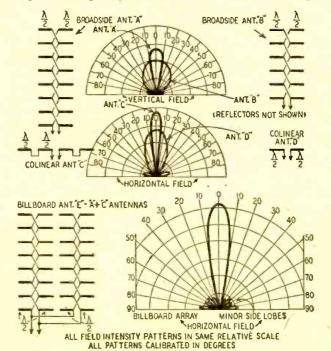
Fig. 2—Showing how characteristics of broadside and colinear arrays are combined in the billboard to give excellent sharpness and gain.
