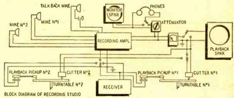
Fig. I-Block diagram of a recording studio with sufficient equipment for professional work.
