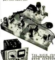
You build MEASUR-ING INSTRUMENT above early in Course, useful for Radio work to Dick up EXTRA spare time money. It is a vacuum tube multimeter, measures A.C., D.C., R.F. volts, D.C. currents, resistance, receiver output.
