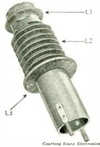
Fig. 5-The high-voltage step-up transformer.
