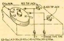
Standard Resistance Current Service Voltage Ohms MaVoltage 1.5 5 300.0 1.2 4.5 150.0 3.6 6.0 100 60.0 4.8 45.0 4,700 9.6 36.0 90.0 9,300 9.7 72.0
