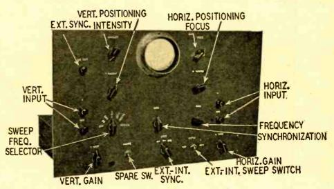
All controls and input and output connections are clearly marked in the photograph above.
