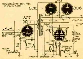
Fig. 6-An "inductive-kick" type of voltage-doubling power supply.
