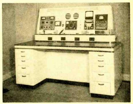
2. One must have a place to perform any operation the radio or other electronic device needs. The space must be large enough to accommodate several radios at once, or a large multiple-unit job, and still have ample room to maneuver. The surface must be smooth, easily kept clean, and nonconducting. Battleship linoleum was chosen as the ultimate in top surfaces.
