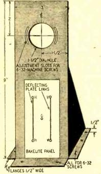
Fig. 3-Rear support of the cathode-ray tube.
