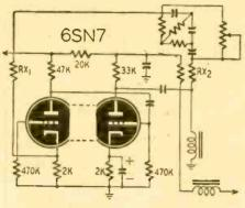
Good results will follow installation of Rx2 whether there is oscillation in the circuit or not. It should then be about 25,000 ohms.
