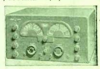
The new NC-173 is a 13-tube superheterodyne model with a calibrated band spread covering the 6, 10-11, 20, 40 and 80 meter amateur bands. Its frequency range extends from 540 to 31,000 and from 48,000 to 56,000 kilocycles for both amplitude modulated phone reception.
