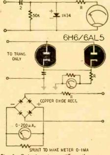
Fig. 3-Output meter rectifiers, three types.
