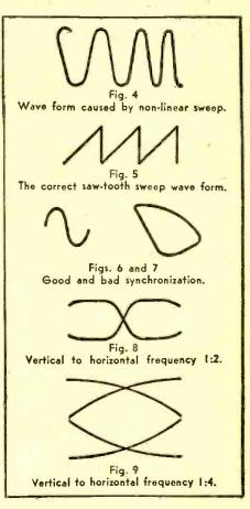
will be given. It is general practice when observing wave forms to use several waves on frequencies of 1,000 cycles and above.
