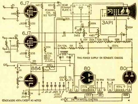
Fig. I—This efficient oscilloscope circuit is simply designed and uses a minimum of tubes.
