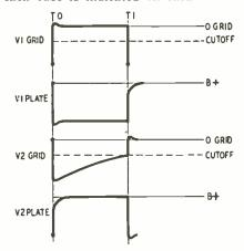
Fig. 6-Analysis of one-kick vibrator action.
