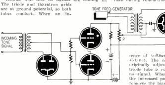
coming signal appears, the output of the fullwave rectifier is applied to the grids as a negative voltage, cutting off both tubes. The triode sence of voltage drop in the plate resistance. The movable contact of P is originally adjusted so that the double-triode tube is cut off during moments of no signal. When a signal does appear, the increased positive potential out of P removes the bias and permits the outgo-
