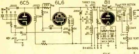
Fig. 1—Schematic of the economy transmitter. Bandswitching is used on the buffer and plug-in coils on the output tank. The 4-prong socket is a male receptacle for the a.c. line supply to the filament transformer, also the low-voltage leads from the pack. The 1,500volt lead is brought in separately.
