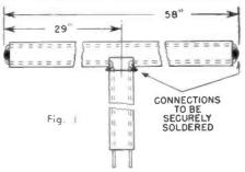
Fig. 1 shows how the antenna is made. The 300-ohm twin-lead transmission line may be type K-1046 (Federal Telephone and Radio) which is especially suitable because of its flexibility, weather-resistance, and very low loss. A 58-inch length of line is shorted at both ends after stripping the insulation as shown. The ends are twisted and soldered. Then one of the conductors
