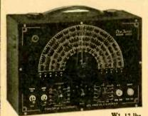
Model 600—SIGNAL GENERATOR: 110-120 volts, 50-60 cycles. RANGE: 165 K.C. to 56 M.C. in 5 bands. AUDIO: 400 cycles, sine wave, 10 volts output. R.F. OSCIL-LATOR: Electron coupled for stability. Ceramic, no drift, coupling condenser. 3 volt R.F. output. \$49.95 Model 600-
