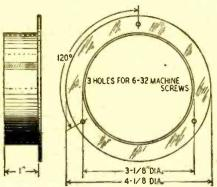
Fig. 2-How the light shield is constructed.
