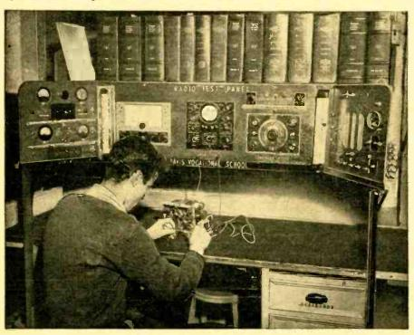
Test panel and service bench constructed by pupils of the Electric Shop, Dover (N.H.) High School. Power panel supplies 117 volts, 6 volts for farm and rural sets, and 2 volts.
