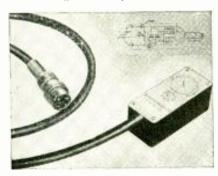
probe used with the Model VM-27 v. t. v. m. It has one-tenth the sensitivity of the standard probe. Consequently, all measured voltages are ten times the indicated values. With the new probe, the Model VM-27 voltmeter has fullscale ranges of 10, 30, 100, 300 and 1000 volts.-RADIO-CRAFT
