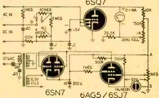
Above—The v.t.v.m. Ranges are—from points I to 4—500 volts, 100 volts, 10 volts and I volt. Below—Carrier-current transceiver.
