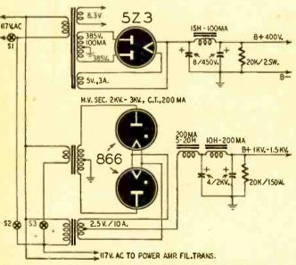
Fig. 3, above—The power supply used for the standby transmitter. Right—Underchassis view shows filament transformer, buffer coils.
