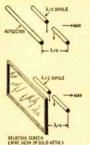
Fig. I—The reflector may be a flat screen.
