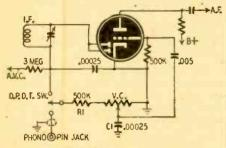
In some sets, the volume control is the entire detector load. In this instance, a 500,000-ohm resistor may be connected in the hot lead of the phono input circuit.
