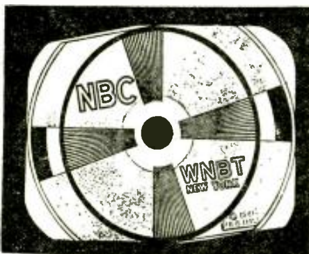
Fig. 7—Deflection yoke is improperly placed.
