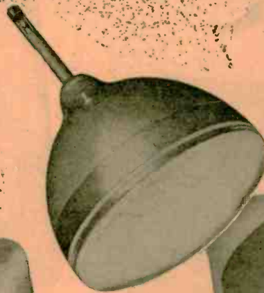
Fig. 10—Large 20-inch DuMont television tube with magnetic deflection and focus. Face curvature radius 30 inches. Picture area 12 \frac{7}{8} by 17 \frac{1}{4} inches. For large screen, direct-viewing telesets.
