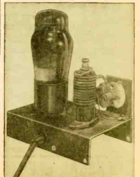
Subchassis holds the transmitting oscillator.
