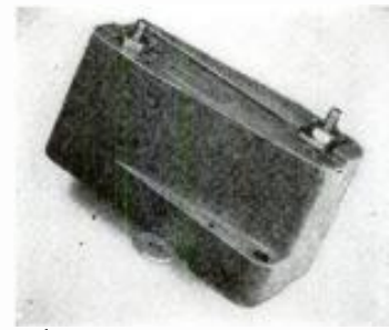
Fig. 14—Lightning arrester protects the set.
