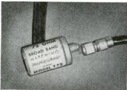
A small transformer replaces matching stubs.
