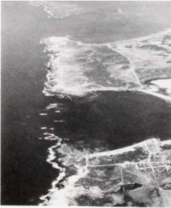
Fig. 23. Waterloo Bay is a curious feature, a circular embayment that has been interpreted in various ways. It is however almost certainly due to the refraction of waves that penetrate the narrow entrance of the feature.
