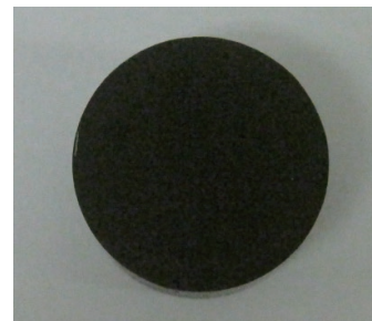
Fig. 1 A fabricated MgB_2 bulk
