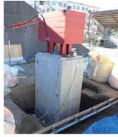
Model pier (simulation of scouring of foundation)
