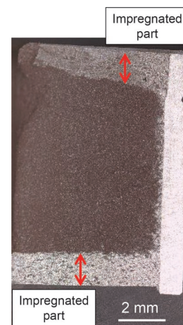
Fig. 17 A cross section of a metal impregnated MgB_2 bulk
