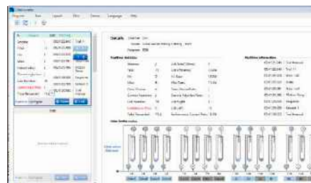
Channel details interface displays key result parameters such as Hit, Miss, False Choice, Correct Rejection, Lick Number, Performance, Correct Rate, and displays the gas cylinder status in real time.
