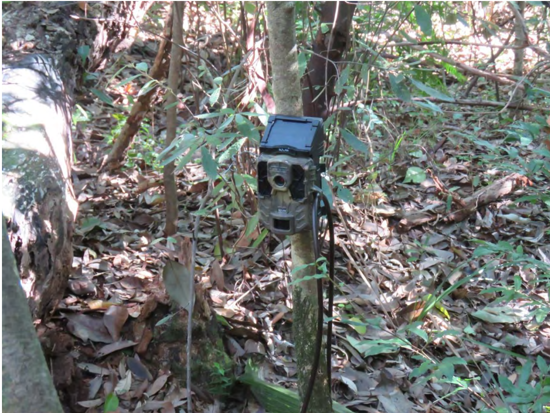
Figure 5 Solar powered cameras with battery backup were deployed for up to 4 weeks in one location. Typically cameras were moved after 7-14 days and bait boxes/lures rebaited after 7 days. Camera at Pembroke Park, June 2017.
