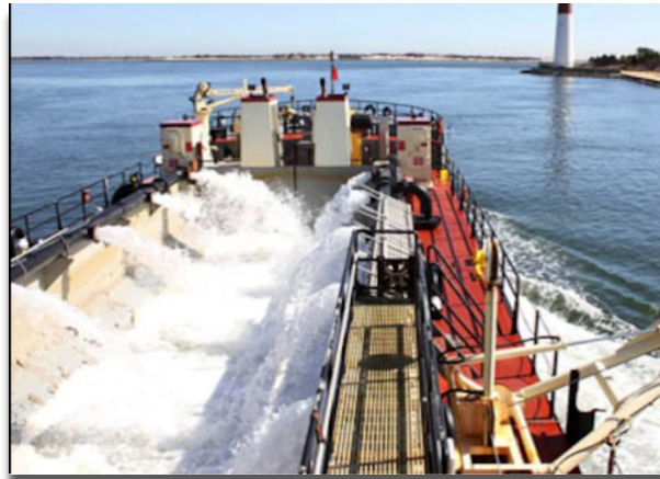
Figure 10 Modified hopper dredge, MURDEN dredging the Barnegat Inlet, NJ in April 2014. Photo by Tim Boyle
