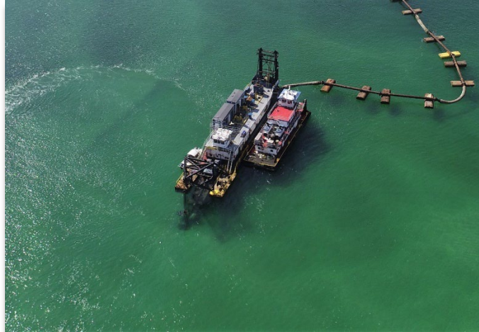
Figure 8 Pipeline dredging by the KELLY in the Gulf Coast Waterway. USACE 2018.
