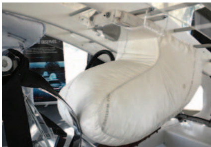
TRW has unveiled its new 'bag in roof' airbag system, which replaces passenger airbags typically mounted in the instrument panel. The new airbag can help cut passenger injuries.
