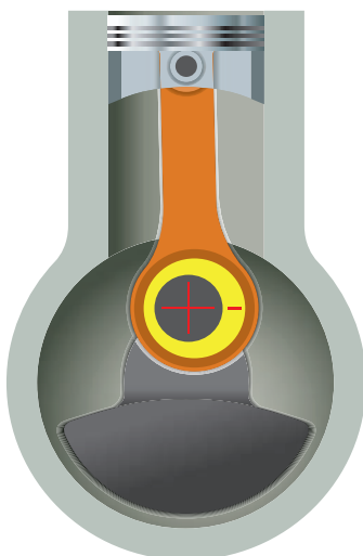
Eccentric at 0 degrees compression ratio 12:1
