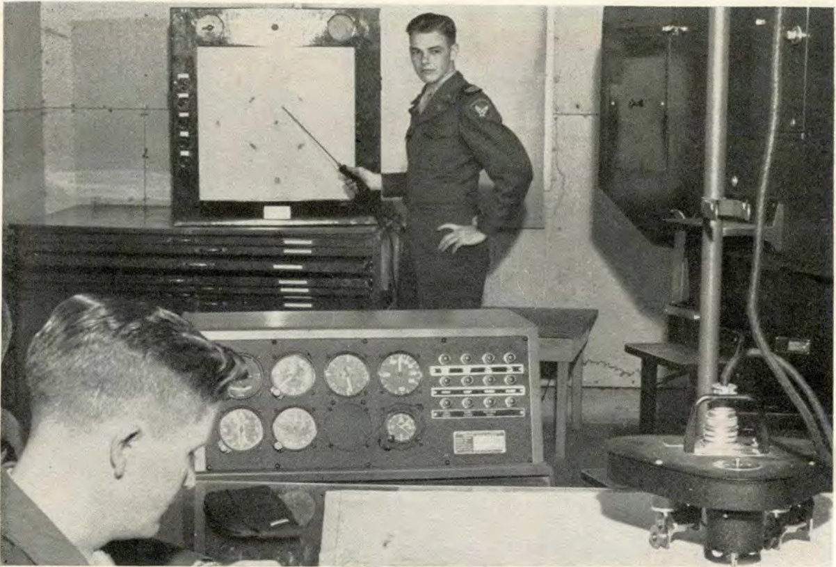
A Cadet demonstrates radio range orientation with a synthetic training device at Barksdale. As the "wand" or pointer in his hand is moved over the station represented on the card, signals duplicating those transmitted by a real radio range are heard.
