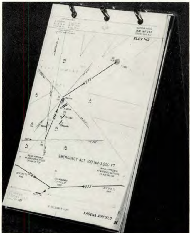
Radical changes have been made on an experimental basis with jet letdown charts. This one fits the pilot's coverall pocket.
