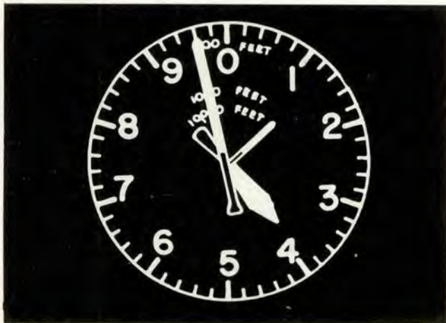
FIGURE 2 Illustration of 1,000-foot error in reading altimeter. Eleven out of 97 pilots read this setting as 14,960 feet.
