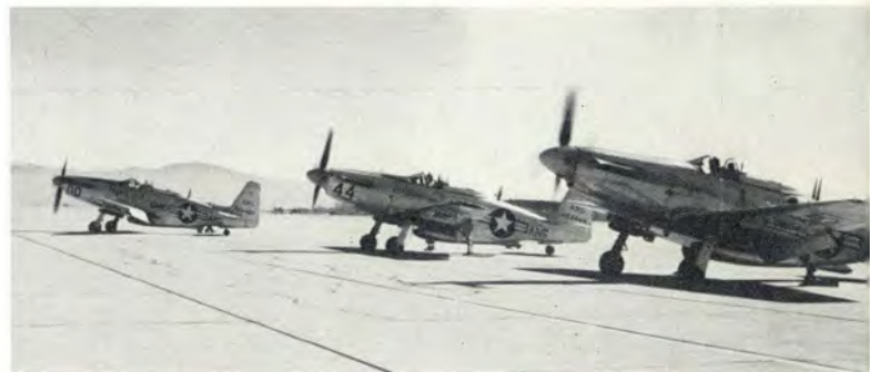
Armament safety had highest priority. Here, guns are charged near end of runway and pointed out across desert.
