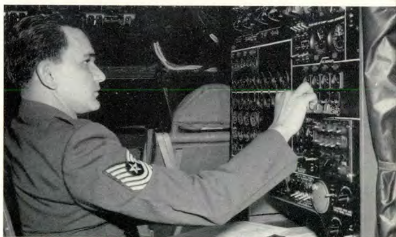
Array of gages and switches before M/Sgt. Frank J. Osborne, of 1252nd Transport Sqdn., is the engineer's panel of a C-97.
