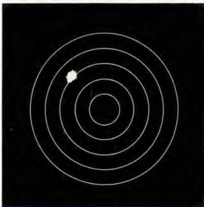
Figure 2B. Tilt could be too high. (No ground clutter reference.)
