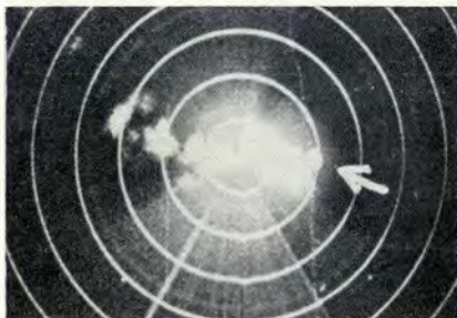
Figure 11, left, pointing finger; center, hooked finger (hail and possible tornado); right, scalloped edges.
