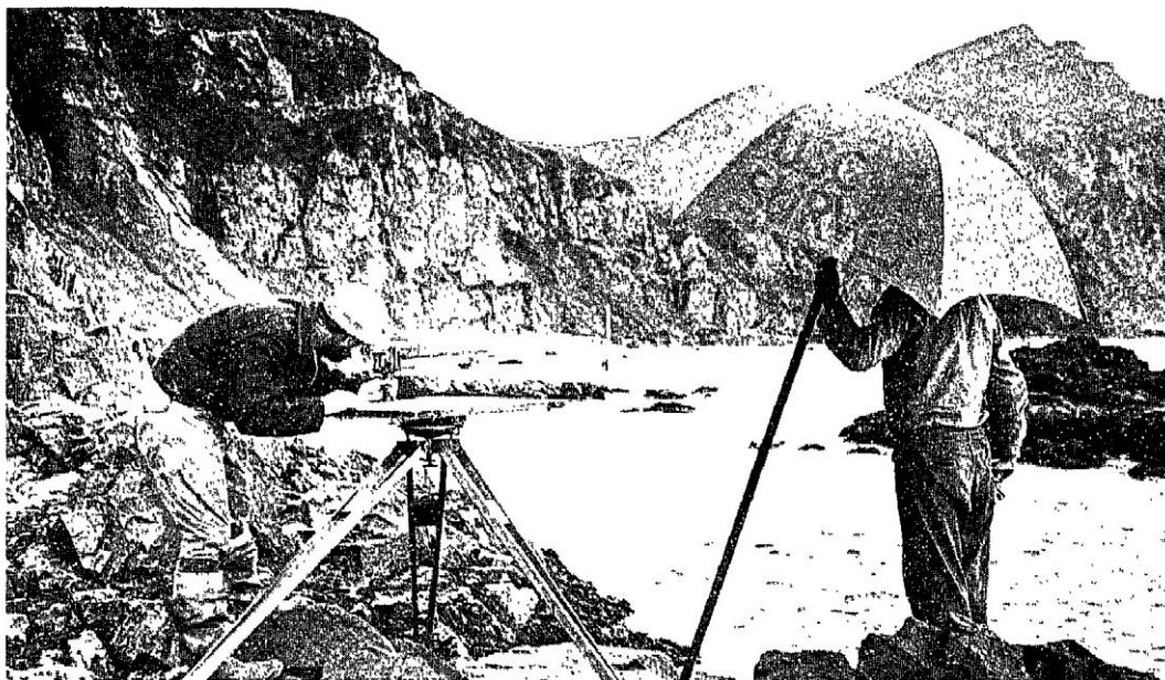
FIGURE 41.—Mapping an Alaska shoreline with the planetable. The planetabler constructs his map as he surveys. The rodman on the point of rocks is holding a telemeter rod and the observer is measuring its distance and direction from the planetable.
