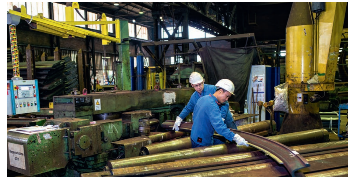
Photo at top: A Peiner Träger GmbH rolling mill. Rolls for various sections are stored at the left, and on the right, the glowing beam blanks drive to the rolls. Right: At the end, the quenched sections are bent in Bochum; an employee checks for the correct curvature
