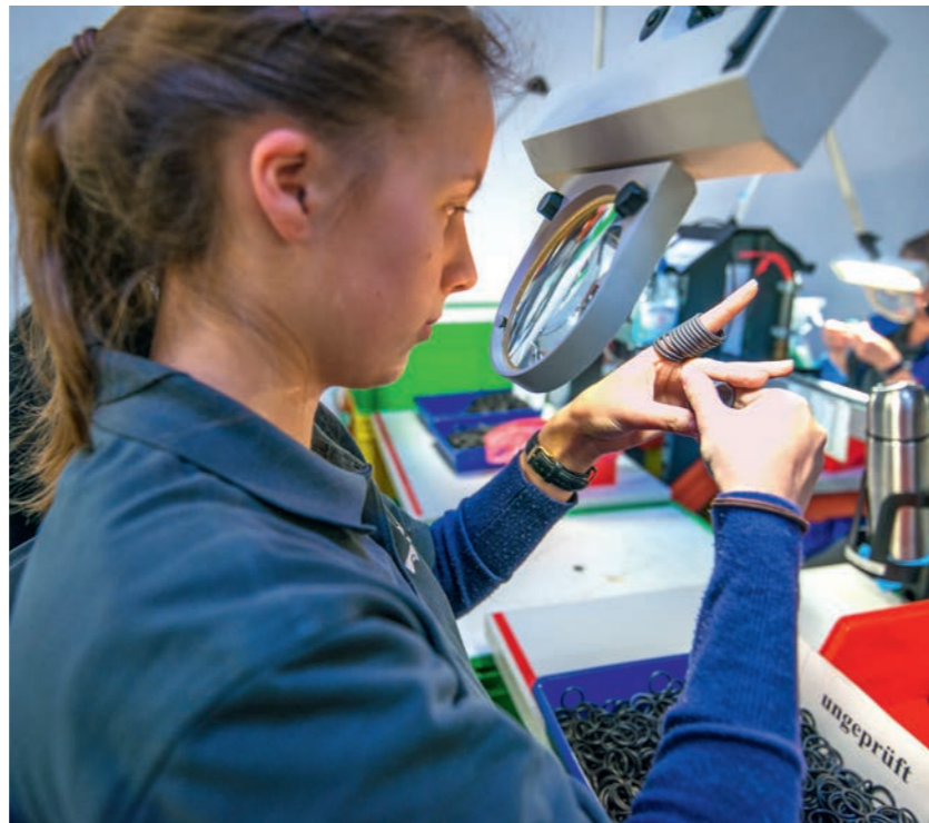
Inspection using a magnifying glass, naked eye and finger: manual quality control in Oberwihl
