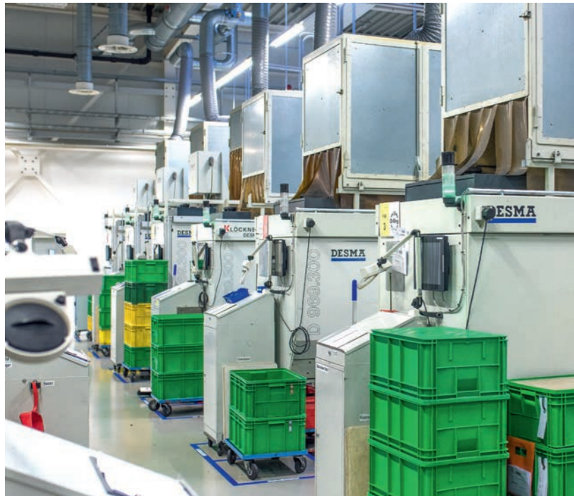
Links: DESMA injection molding machines at Freudenberg: the elastomer compound is injected into the mold at pressure levels of up to 3,500 bar. The compound is heated to approx. 180 degrees and as liquid as water. Right: After pressing the O-rings have to be deburred
