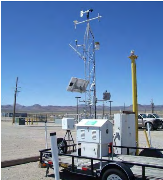
Figure A-1. Station 400, located near the Range Operations Center, includes an array of devices to measure radiological and meteorological conditions
