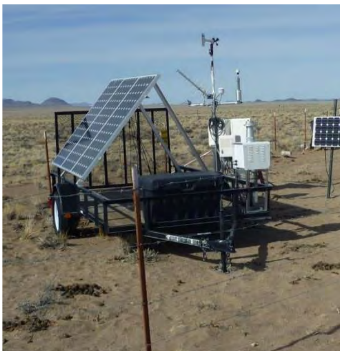
Figure A-3. Station 403, located along the south fence that bounds the Clean Slate III contamination area, includes a solar-powered air sampler and meteorological tower
