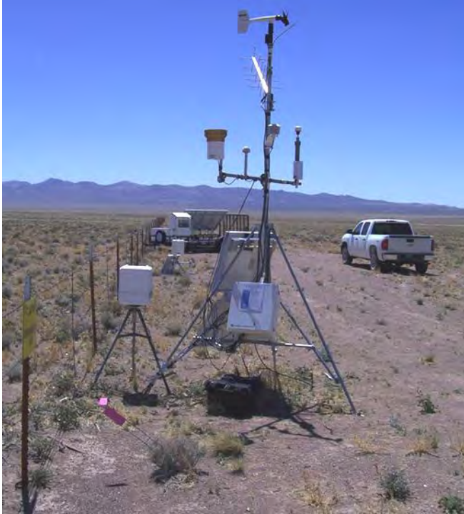
Figure A-2. Station 401, located along the north fence that bounds the Clean Slate III contamination area, includes a solar-powered air sampler, saltation sensor, and meteorological tower (background, center, and foreground, respectively)
