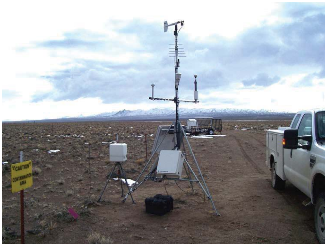
FIGURE 1-5. The Station 401 portable meteorological tower and instrumentation are located on the fence on the north side of Clean Slate 3.
