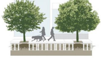
Suspended pavement with sufficient soil volume for trees to develop deep roots
