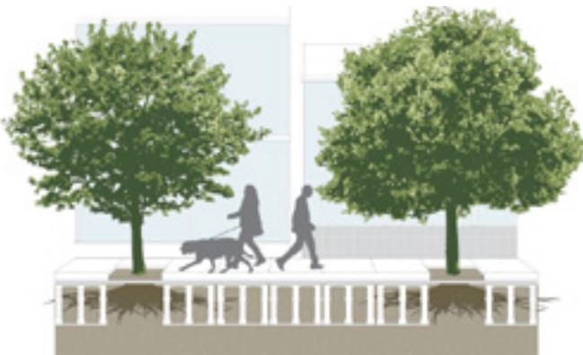
Suspended pavement with sufficient soil volume for trees to develop deep roots
