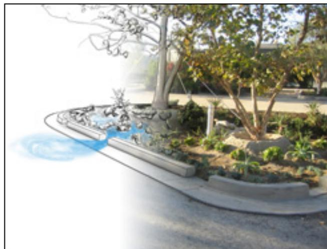
Bioretention with Infiltration
