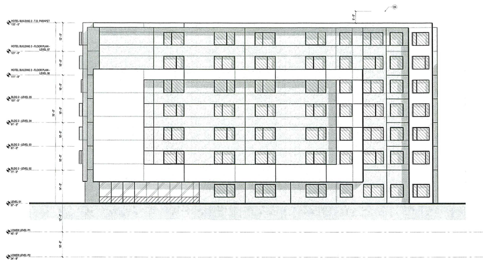
1 HOTEL BLDG 2 - WEST ELEVATION SCALE: 1/8" = 1'-0"
