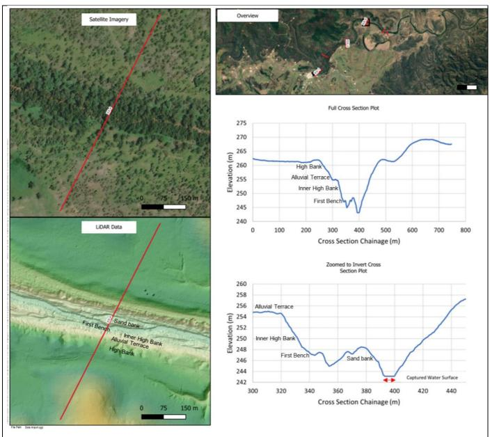
**Figure 21**: Profile of the Dawson River at site XS-4, approximately 2.5 km upstream of the watercourse and waterhole discharge point. Clockwise from lower left: a representation of bank topography based on LiDAR imaging; satellite imagery around this transect, an overview indicating the location of the cross-sectional transect; a graph of elevation across this transect; and a larger scale graph of the cross-section between the high banks (Figure provided by AECOM).
