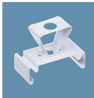
ZTX400 SMS Cable suspension bracket for suspending the TTX400/410 sections from steel cable M1.5. Integrated adapter allows easy, toolless adjustment of the mounting height. Steel cable can be ordered separately with accessory ZTX400 WIRE (10 m).
