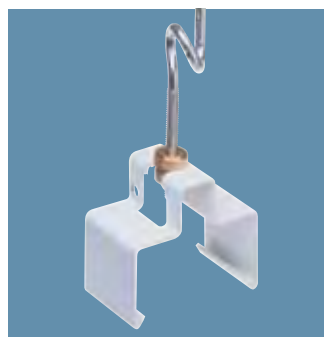
ZTX400 CB Chain bracket for suspending TTX400/410 sections from chains or steel cables. Includes adjustable suspension hook.
