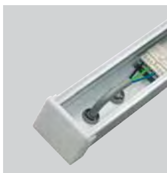
TTX400 TL-D/TL5 trunking Alternative, more aesthetic mains connection, using a standard electrical connector. Knock outs in trunking and end caps enable the mains wires to enter the trunking. Dedicated trunking e.g. TTX400 491 CU7 with knock outs. Kit: electrical connector, end plate and 2 cable glands e.g. ZTX400 EP-CU7.
