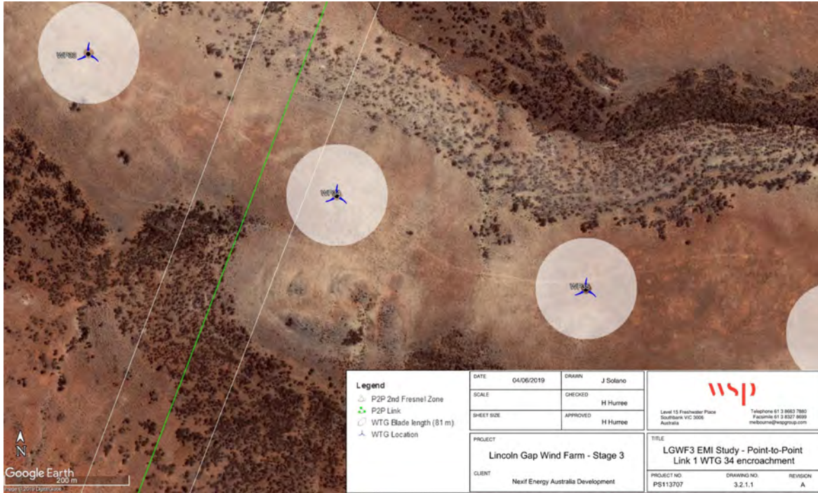
Figure 3.3 Point-to-point Link 1, WTG 34 encroachment
