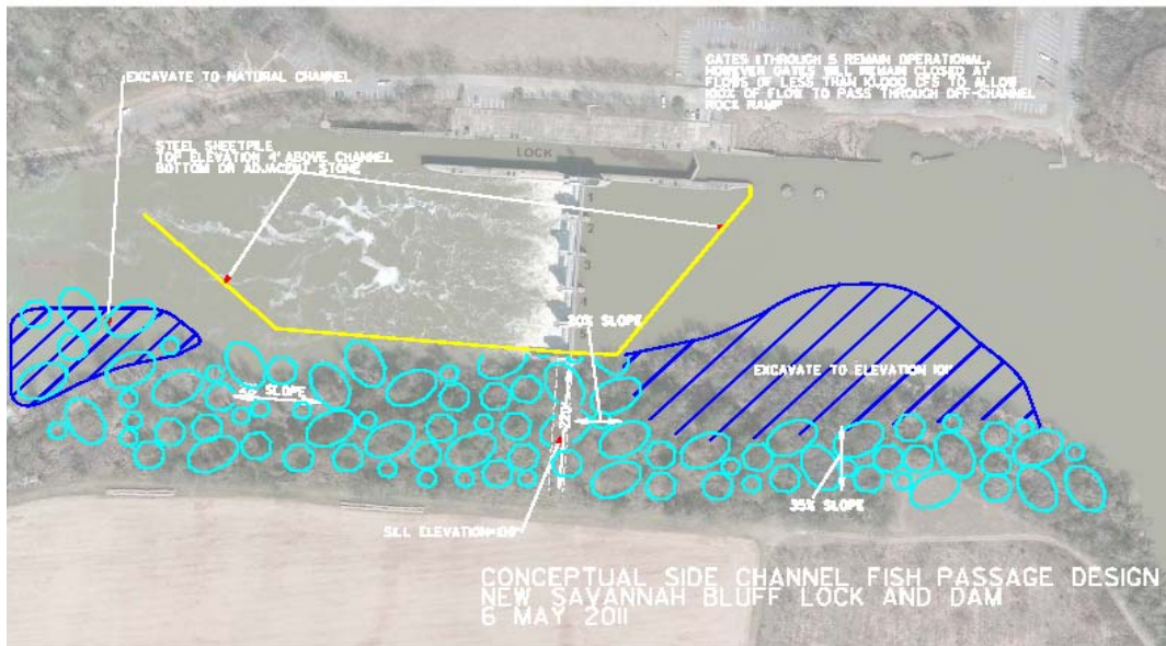
Figure 7. COE-proposed Off-channel Fish By-pass Design at New Savannah Bluff Lock and Dam
