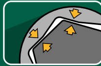
Sockets feature off-corner loading
