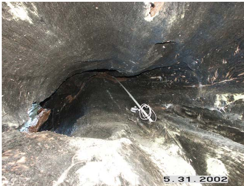
Figure 8. Temperature probe installation inside basal hollow. Lower probe is visible. Interior probe is on end of pole inserted high in the hollow.
