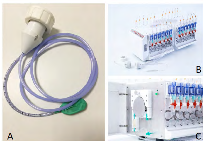
FIGURE 1. A) Manometric probe. B) 24 channels water perfused system (Alacer Biomédica). C) Perfusion pump.
