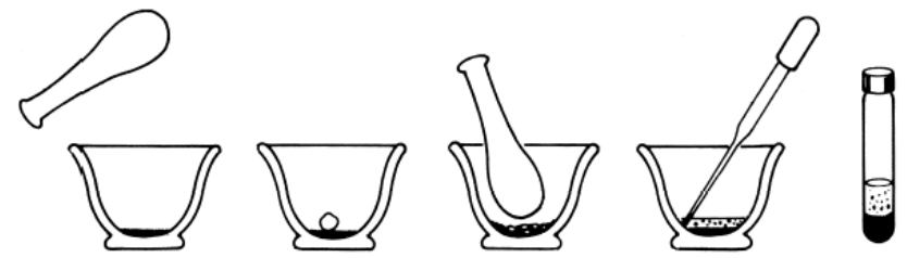
Figure 3.13.1-2 Illustration of mortar-and-pestle method of homogenization of tissue.
