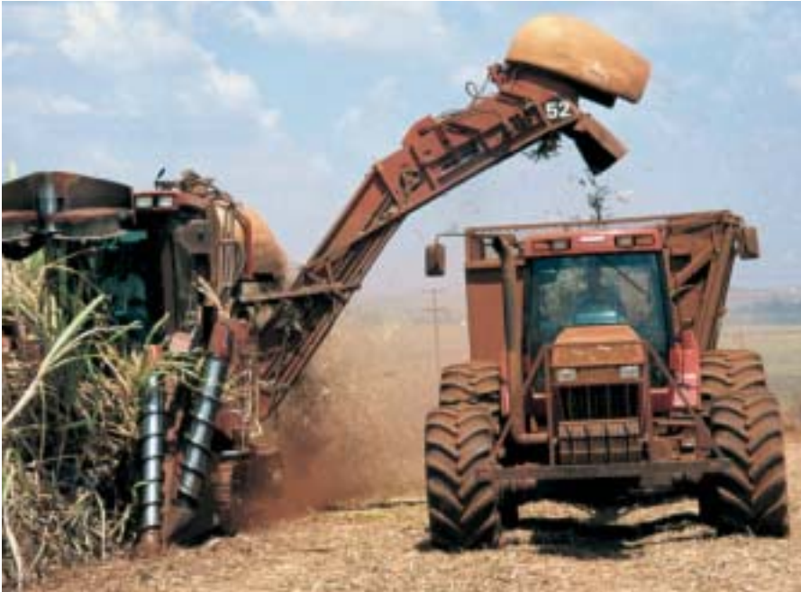
Sugar cane harvesters with Scania engines in Brazil can harvest one tonne of cane per minute.
