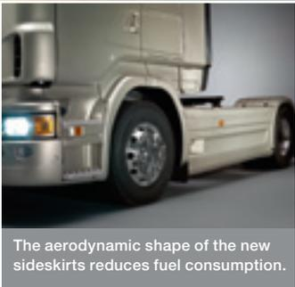
The aerodynamic shape of the new sideskirts reduces fuel consumption.
