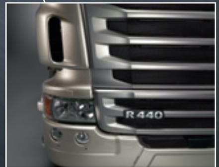
The grille has substantially larger openings between distinct horizontal bars. This underscores a Scania's identity while admitting more air to the radiator and into the engine compartment.
