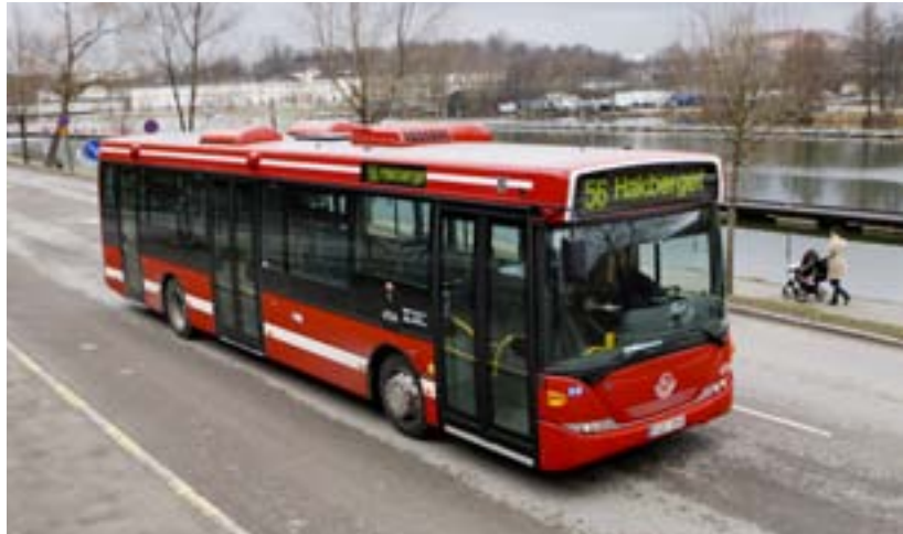
Like its tourist coaches, Scania's city and suburban buses are based on modularised components. This is also true of the bodywork, which can be tailor-built according to customer requirements in many different configurations, for example as a low-floor bus, a low-entry bus, or a two-axle, three-axle, double-decker or articulated bus with the help of the same set of components.
