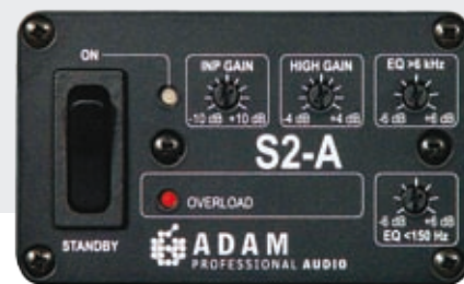
Control panel S2A
